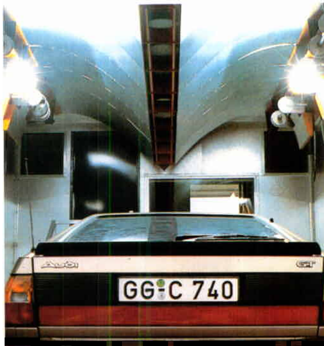
10 Solar simulation: HMI (1200 W – 4000 W)
