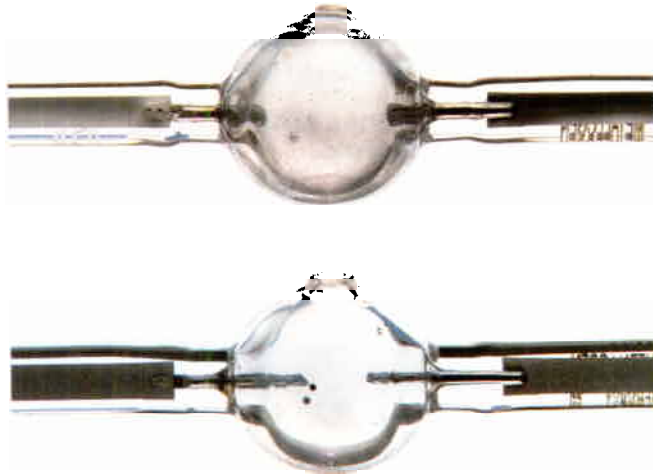
74 Melted electrodes (top), new lamp (bottom)
