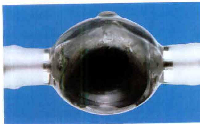
76 Result of a leak in a lamp with no outer bulb
