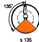
56 Permissible operating positions for HMI, HMP, HTI, HSR and HSD lamps
