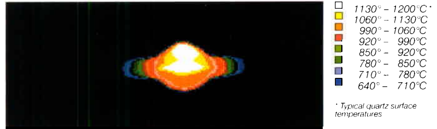
b : Discharge tube in the vertical position
